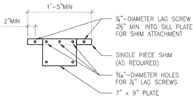
CONNECTION WHEN SHIM SPACE EXCEEDS ¾" INCH WIDTH UP TO 1½"
