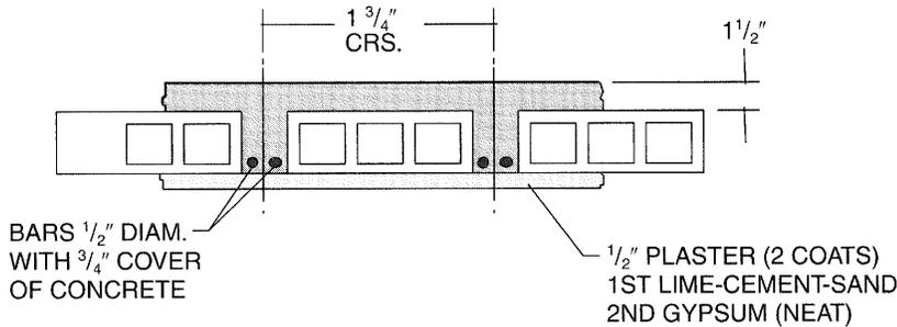
1. A generalized cross section of this floor type follows:
