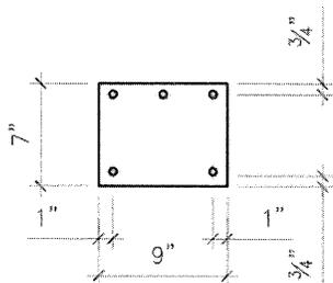
HOLE DIAMETER SHALL NOT EXCEED CONNECTOR DIAMETER BY MORE THAN 1/16"
