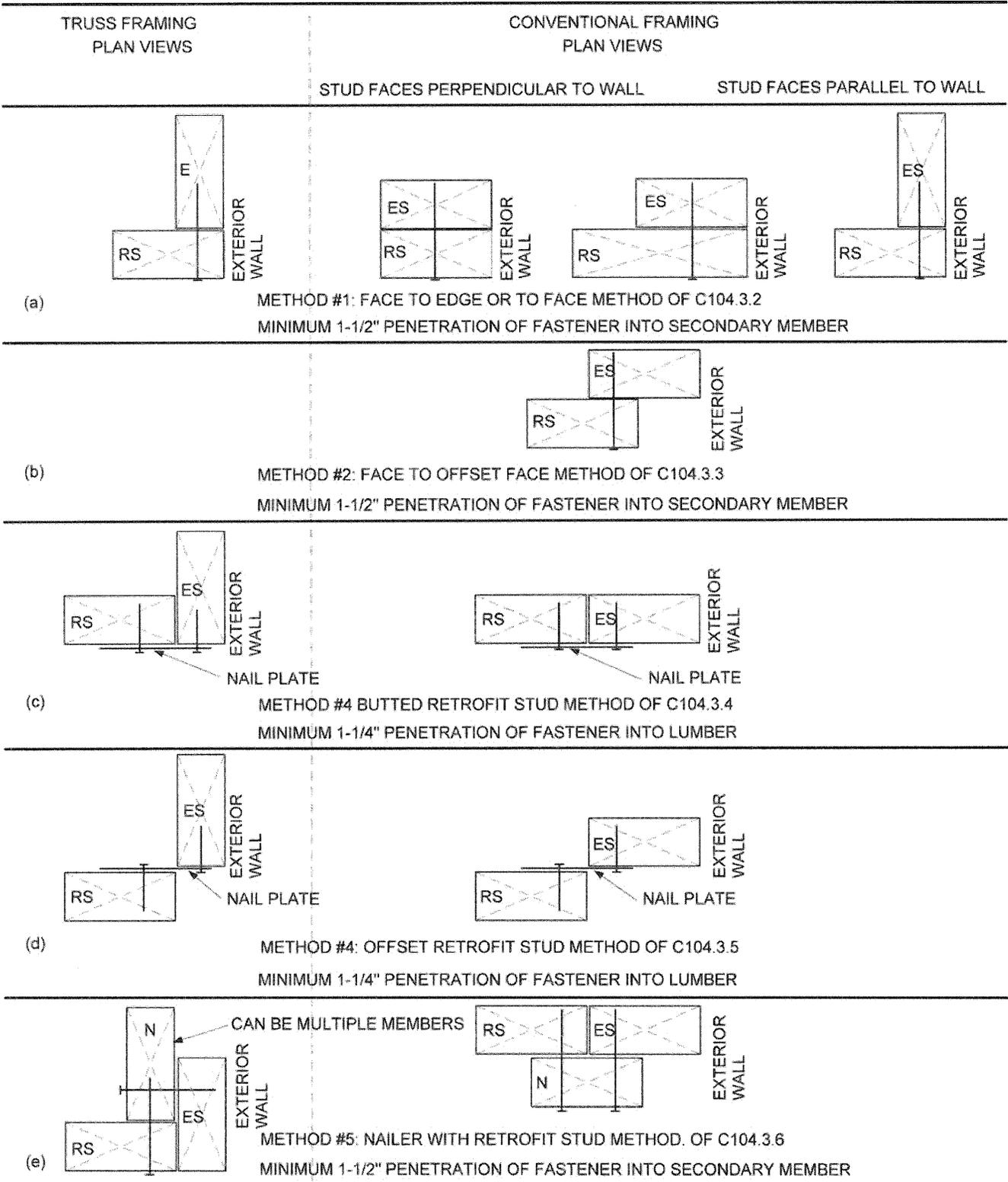
THE FIGURES DO NOT REFLECT THE NUMBER OF REQUIRED FASTENERS OR SHOW HORIZONTAL BRACES OR STRAPS. FASTENERS SHALL BE PLACED MAXIMUM 6" ON CENTER AND A MINIMUM OF 2-1/2" FROM ENDS. 3" FASTENERS CAN BE INSTALLED FROM EITHER SIDE OF LUMBER AS LONG AS THERE IS 1-1/2" FASTENER PENETRATION. ES INDICATES AN EXISTING STUD. RS INDICATES A RETROFIT STUD. N INDICATES A NAILER.
